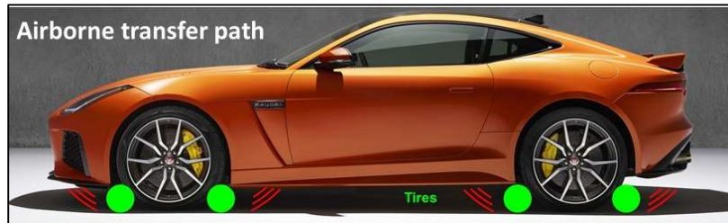
Figure 3: road noise – airborne path
