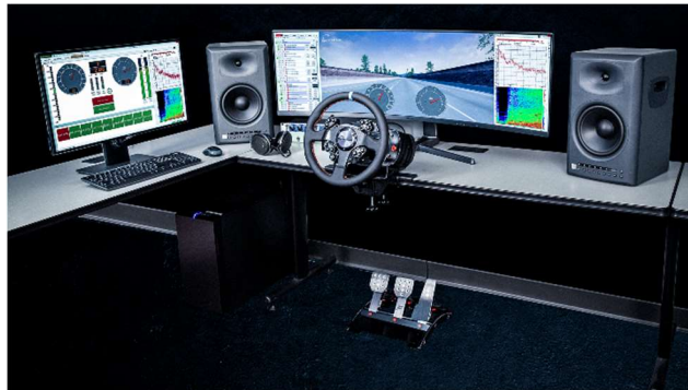
Figure 1: driving simulator for NVH
