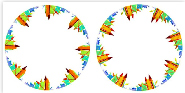
FIGURE 3 Reduction of the loads to the stator teeth at 2 time steps t=0.0s (left) and t=0.00312s (right).
